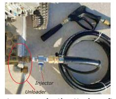
Foam injector conveniently attaches after the pump/unloader on your pressure washer
