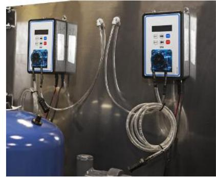
Dual peristaltic pump assembly, RC-0021-0002
