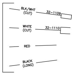
TAPE ENDS CLOSED TO SEAL WIRES (2) PLCS
