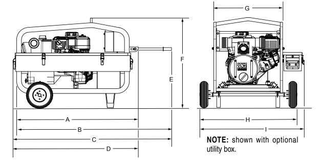
Figure 1. QP3Ti Dimensions
