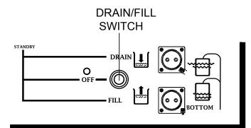
Figure 13. DRAIN/FILL Switch
