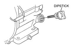
Figure 6. Engine Oil Dipstick (Removal
