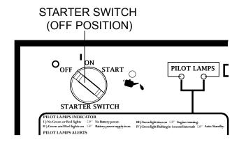
Figure 16. Starter Switch (OFF)
