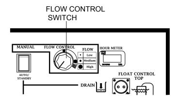
Figure 12. Flow Control Switch
