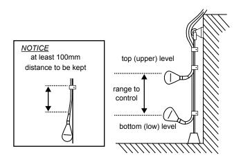
Figure 15. Float Switches
