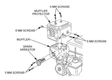
Figure 21. Spark Arrester Removal
