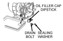
Figure 19. Engine Oil (Draining)
