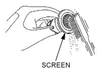
Figure 22. Cleaning The Spark Arrester
