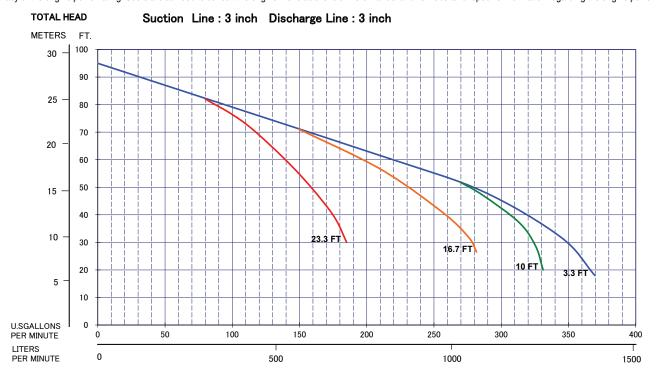
Figure 2. QP3Ti Performance Curve
