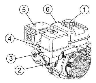
**Figure 4. Engine Controls and Components**
