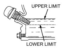
Figure 7. Engine Oil DipStick (Oil Level
