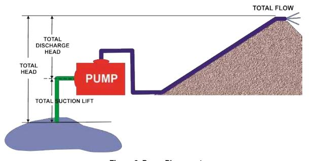
Figure 8. Pump Placement
