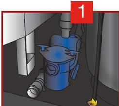
Surface-mount sump pump located behind the carbon filter
