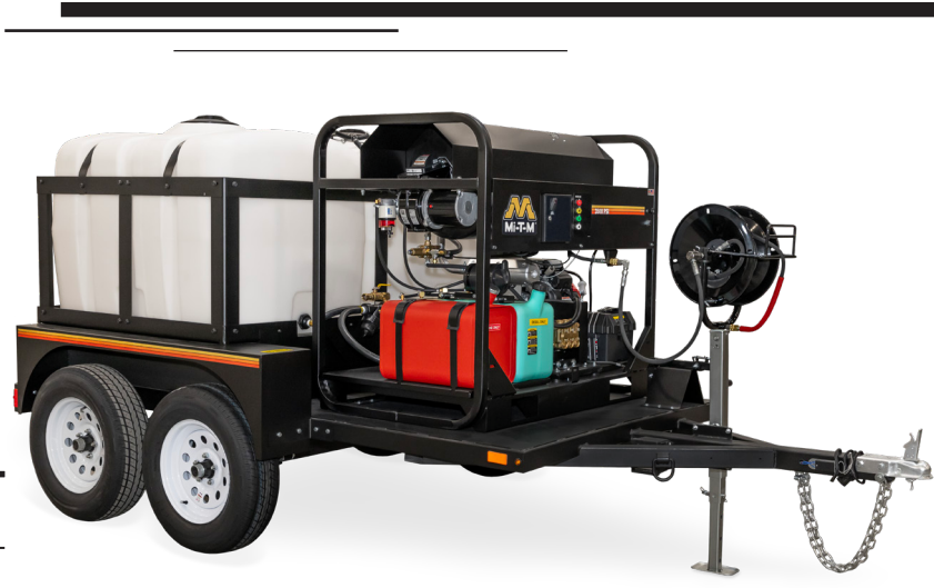
AW-9000-0004 Dual-Axle Trailer Shown with HS-3505-1MGH hot water pressure washer and high pressure hose reel, TX-0001
